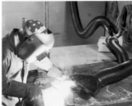
In the same application, the fumes and smoke are ducted completely out of the work area by the Power Cat and its duct and intake accessories.
