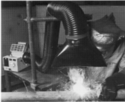
Welding galvanized pipe generates zinc oxide fumes and smoke that are efficiently removed by the Power Cat.
