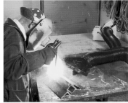
The Power Cat removes and exhausts fumes and dense smoke generated by heavy, iron-powder electrodes.
