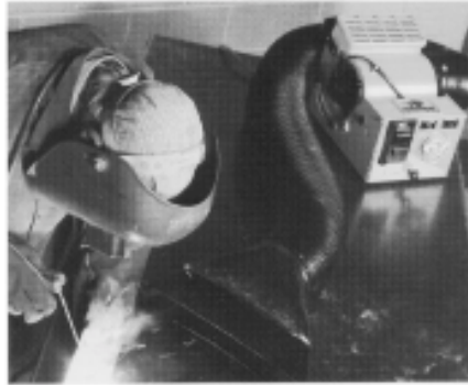
The Power Cat quickly exhausts harmful toxic oxides produced by the use of low hydrogen electrodes to weld stainless steel, nickel, chrome, etc.
