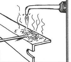
Position the parts and heat the metal indirectly until the flux boils and turns clear.
