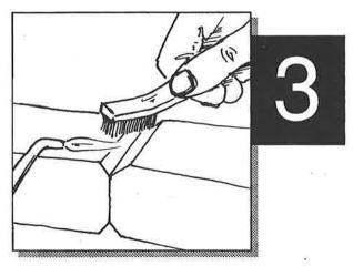
Brush tinned surface under heat, thoroughly filling open pores. This constitutes welding without fusion.
