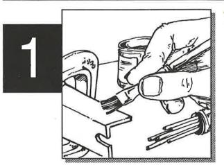
Clean the metal thoroughly. Stir flux well, then apply flux to both surfaces.
