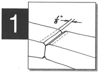
Vee the broken edges to about 45°. Clean the surface of any plating or scale back from the edges of the vee 1/8 inch.
