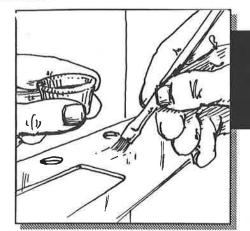
When using solder with #1 low temperature liquid soldering flux, apply flux to the cleaned area, heat, and apply solder. Use low heat with torch or soldering iron.
