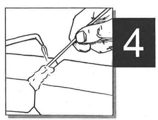
With sides thoroughly tinned, flow enough rod to fill the Vee. Be sure the filler metal fuses with the tinned surface without melting the base
