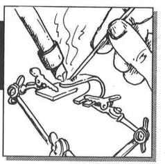
When using flux-cored solder, any common soldering technique can be used. Use low heat with torch or coldoring iron
