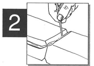
Heat the metal until it starts to flow. Turn the flame parallel to the surface. Hold the metal at this heat with the side of the flame. Heat the rod to the same temperature.
