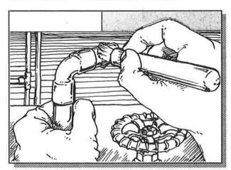
The plastic-coated fiberglass strands of the Aladdin #37 Fiberglass Brush are excellent for friction-tinning aluminum, and clean other metals readily. Makes an excellent flux brush, and in preparing metals for heliarc welding nonmetallic material.
