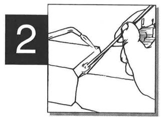
Heat the metal hot enough to flow the rod without the aid of the flame, thoroughly tinning the surface.
