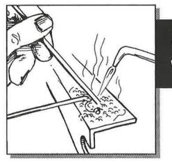
Immediately apply solder and melt quickly, putting the heat directly on the area to be soldered. Solder will creep into the joint.
