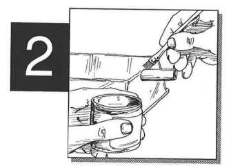
Apply the appropriate flux to the metal and heat.
