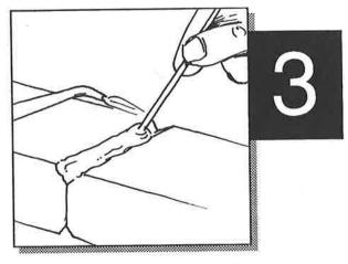
With both base metals and welding rod at the same temperature, touch the rod to the break. The rod will flow into the vee, thoroughly fusing. Repeat this procedure until the break is completely filled. Be sure to kick the rod into the weld to break down skin resistance as the filler rod will lay on the surface and will not fuse if only heat is applied.
