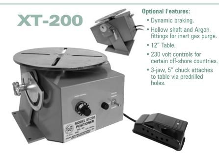
Atlas positioners can help boost production on hard to handle jobs requiring circular welding (small spheres and pressure vessels; flange-topipe; pipe-to-pipe; etc.) Heavy duty grounding circuit allows use of stick electrode, MIG or TIG welding processes.
