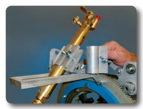
Now standard on all H&M's Saddle-Type Beveling Machines, the Adjustable Torch Holder, the Out-Of-Round Attachment and all Shape Cutting Attachments, the Solid Torch Holder provides greater cutting accuracy, efficiency and strength. A single thumbscrew secures the torch instead of hose clamps. A cotter pin makes the thumbscrew captive to the torch holder, allowing easy removal or replacement of the torch. Precise and simple to use, the Solid Torch Holder means solid performance.
