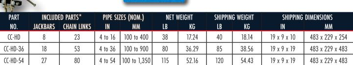
NOTE: All pipe clamps are ONLY designed for aligning pipe ends during the welding or tacking process. DO NOT use the clamp (s) to support any weight of pipe and/or fittings in any situation. DO NOT use the clamps with shims, wedges or cheaters.
