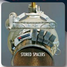
In the past 12 spacers were required. The saddle of each H&M machine and the four cuboids allow four specific pipe sizes to be cut. Each side of every cuboid spacer is clearly stamped to ensure cutting the correct pipe size. When not in use the cuboid spacers are securely housed on the back of the saddle. It's a no-lose proposition in time-saving productivity!
