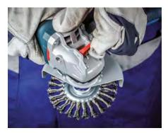
Release the brush by using the lever.
